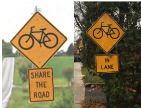
EXAMPLES OF SHARE THE ROAD SIGNAGE. THE ONE ON THE RIGHT IS RECOMMENDED.
